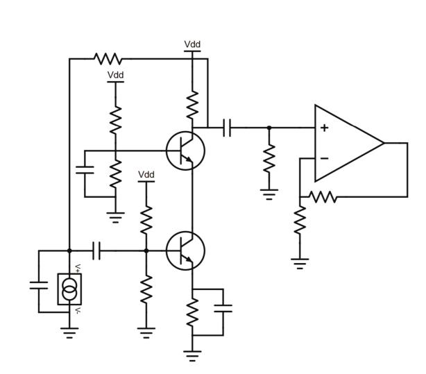
Front-end electronics for the photoreceiver amplifier must provide a flat frequency response in the range of interest (10 MHz to 30 MHz) and a low contribution to the noise budget in order to ensure a shot-noise limited operation.
